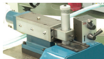
Hydraulic over-head wheel dresser (84AHD).
